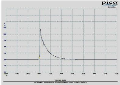
achieved easily using the same capacitor details as before. Note that this does not include the battery voltage.
