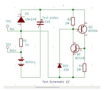
So whatever net charge is returned through R1 will be essentially "profit" harvested from the mechanical input. Therefore the overall effect of the design is to convert mechanical energy into a charging current that can either charge a battery or maintain it's charge when supplying a load circuit.
